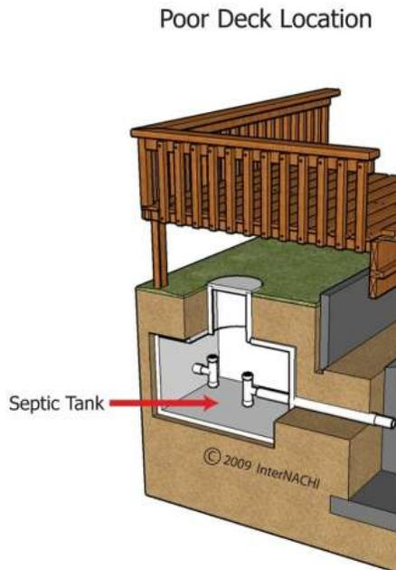
Access ports may be visible and exposed at ground level. The access ports should not be more than 12 inches below the ground surface.
