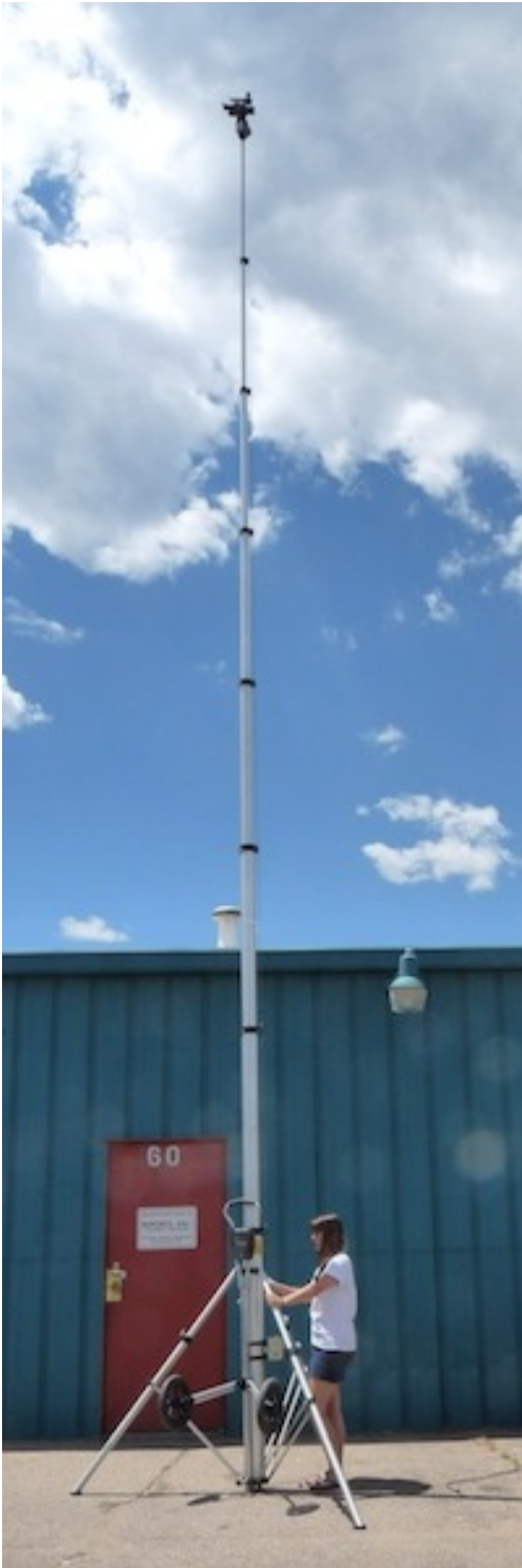
The tripod extends up to 35 feet. Some are available that extend up to 70 feet.
