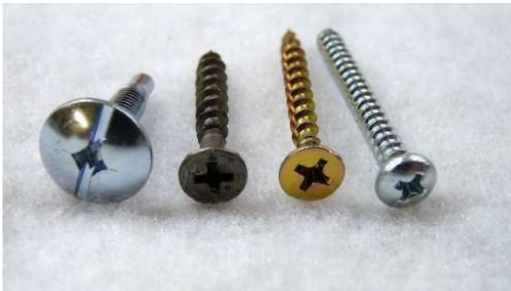
The photo above shows (from left to right) a proper dead front or panel cover screw, along with three improper but commonly used screws, including a particleboard screw, a gold deck screw, and a machine screw.
