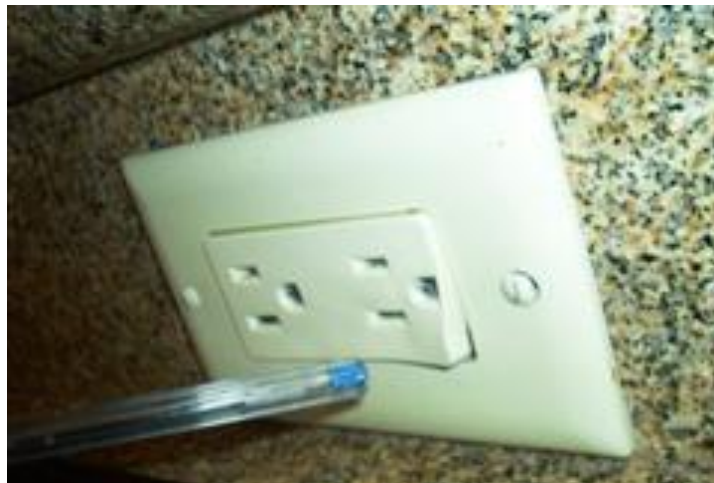
above: a melted outlet
