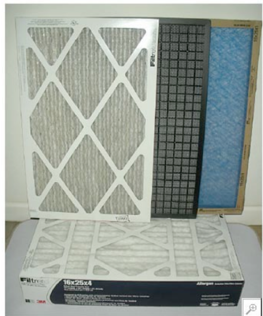
On the left is a 1-inch MERV 8 pleated filter, which is similar in appearance to all other 1-inch pleated filters tested. In the middle is the washable MERV 8 WEB filter, and on the right is a typical fiberglass filter that was used for comparison. At the bottom is a 4-inch MERV 12 pleated filter.
