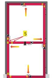
*Tip:* Fit the frame so that it is tight enough to remain standing in the doorway, but can be removed with a slight pull.
