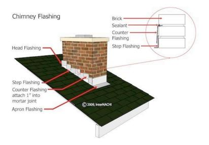
This illustration shows counter-flashing installed correctly. It fits into grooves cut into the mortar joints. After the counter-flashing is installed, the grooves are sealed with an appropriate sealant.
