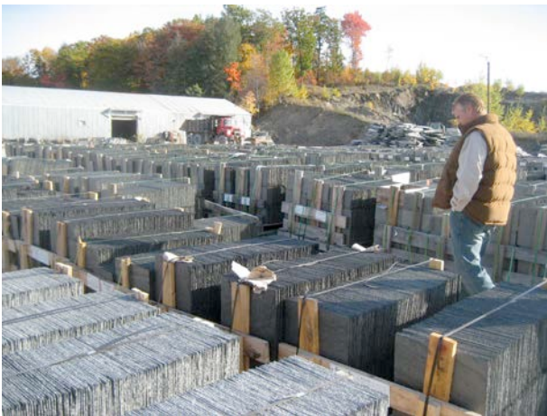
Finally, slates are loaded onto pallets to be trucked to the jobsite.
